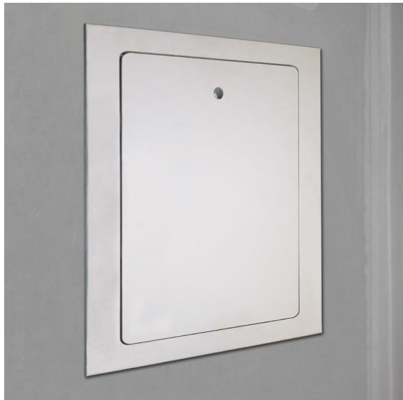
Trappe T EI30 Vac, E30-EI30, 34 (-1 ; -2) dB, 400×400 mm (TA-100)
